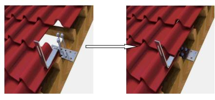
Partially open the tile and fix the hook to the purlin of the roof.
