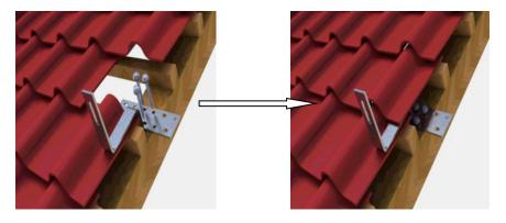
Partially open the tile and fix the hook to the purlin of the roof.
