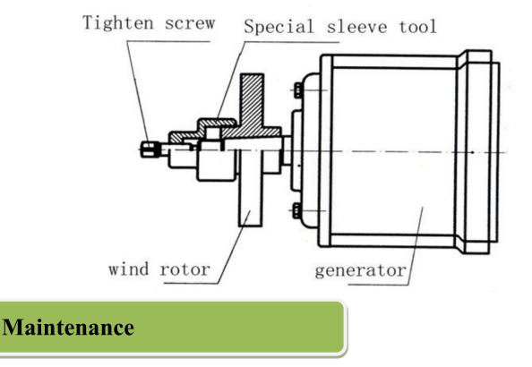
After 20 years of service the blades MUST be replaced – even if there is not apparent damage. The
